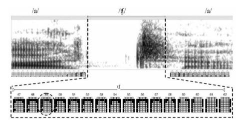
**Figure 2.** Segmentation and annotation criteria illustrated with the nonsense word /atʃa/ produced by the speaker F1. The frame of maximum EPG contact is encircled (ACoG is 6.5 and the amount of contact is 40%).
